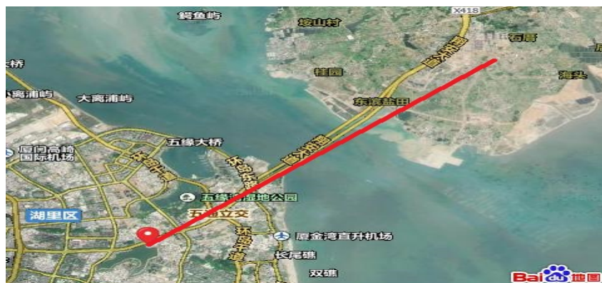
Xiamen \pm 320\text{kV}/1000\text{MW} VSC project, cable length 21km, commissioned in Dec. 2015
