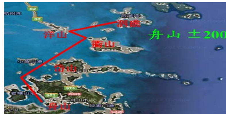
Zhoushan \pm 200\text{kV}/400\text{MW} 5-terminal VSC project, cable length 294km, commissioned in Jun 2014
