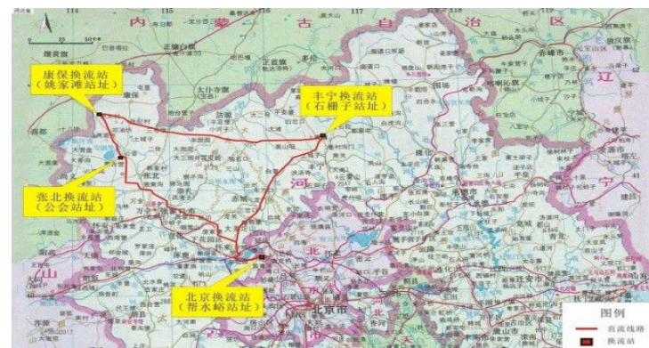
Planned Zhangbei \pm 500\text{kV}/3000\text{MW} 4-terminal VSC projects, 500km OHL, 4x500m trial cables, project for 2022 Beijing Winter Olympic.
