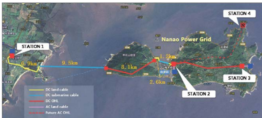
Nan' ao \pm 160\text{kV} , 200MW 3-terminal VSC project, cable length 35km, Commissioned in Dec. 2013
